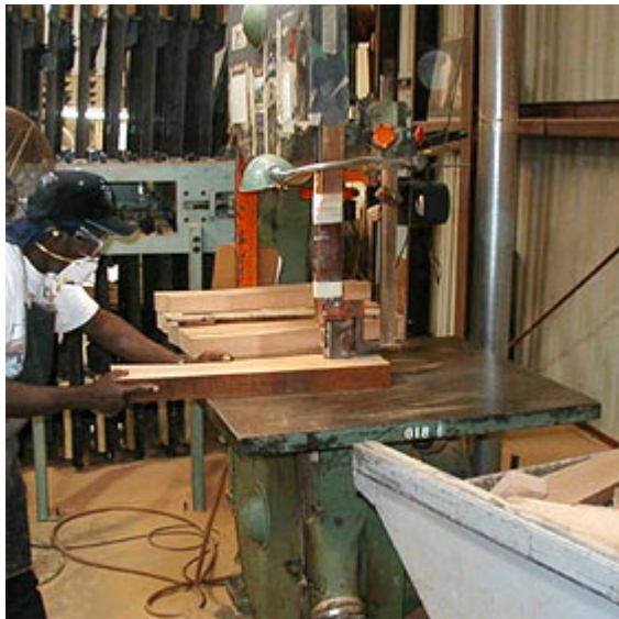
A guitar craftsman cuts the neck of a Les Paul guitar from sustainably harvested mahogany, at the Gibson factory in Nashville, Tennessee. Photo courtesy Gibson.
