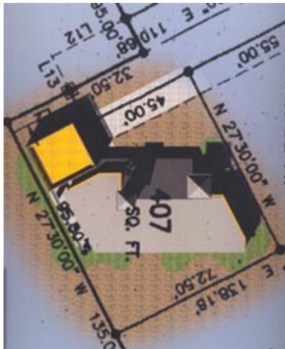
The passive solar residence, superimposed over the plot plan, showing true southern orientation. Graphic by Rich Michal.
